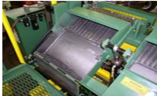
2 Nail Pans hold 100 lbs. of loose nails and have quick unloading.
