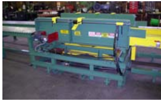
All hydraulic Stacker. GBN uses this on all its systems.
