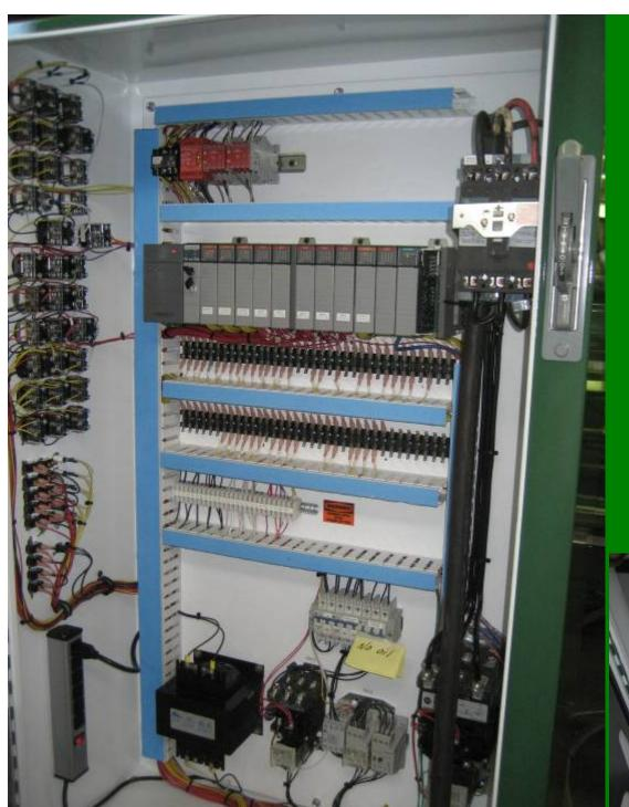
The brains of all GBN System. Large roomy enclosures using all Allen Bradley Components including an Allen Bradley Programmable Controller with enclosure circuit breaker, cut off and adjustable off line voltage starters. A GBN is ready for any three phase voltage right out of the box. It even has a machine tool transformer for the 120 volt AC control circuits. Bringing power to a GBN is very easy.
