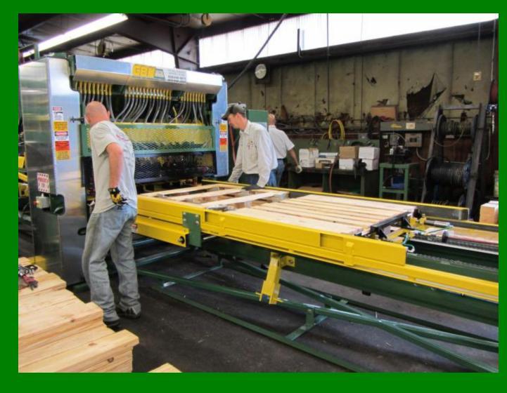
When you choose the option of making block pallets on your GBN Patriot System, top deck nailing is included with ejection system.
