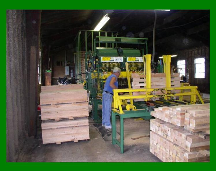
**Optional** Setup to make Block type pallets. Pre made top decks are no longer needed. The Patriot nails it all in one pass, Correctly.
